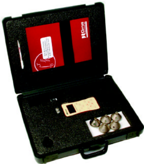
CK110/5 Measurement Kit, showing the five doseBadges mounted on the 5-way charger.
