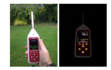
Most environmental noise surveys demand the use of a Type 1 Sound Level Meter that can make repeating measurements, such as the 5 minute LAeq and L90 (background noise).
